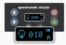
Digital counter, battery level symbol and control mode displayed on screen.
