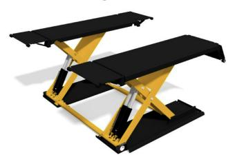
Extra low rise electrohydraulic lift with min. travel 96 cm and double platform. Platforms connected by double torsion beam for perfect synchronicity and levelling.
