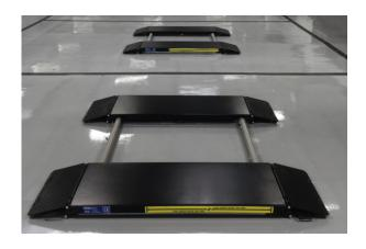
pin, no maintenance required, High- sliding and self-lubricating polyethylene sliding pads. Lowering speed control with compensation valve. "Hold to run" 24V Control.
