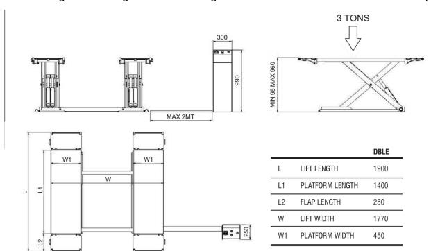
Capacity 3000 kg Power Unit Kw 1,1 400V 3Ph 50Hz Total weight 500kg Lifting height max 960 mm Up-Down Travel speed 20/20sec Equipped with 4 flap run- up ramps Hoses covered with anti-blast sheath Kit of 4 rubber pads h 20mm
