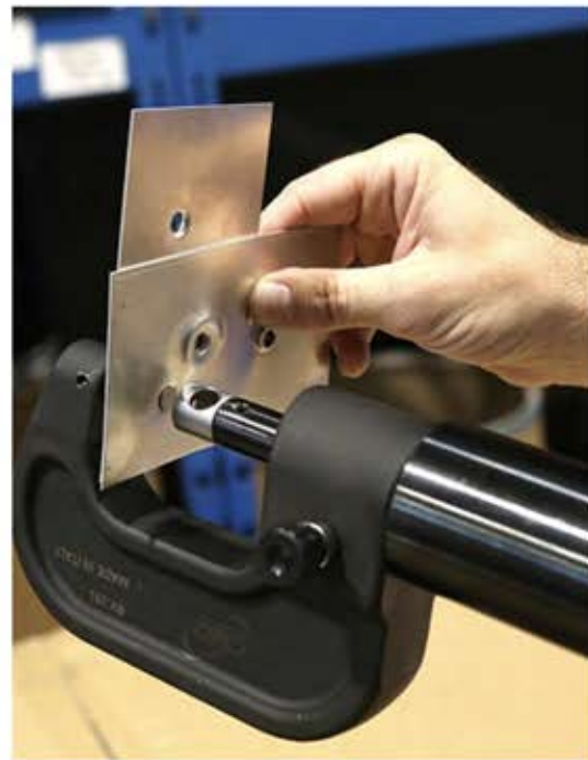
CMO RV/EP02 Riveter easily joins sheet metal or removes rivets already installed.
